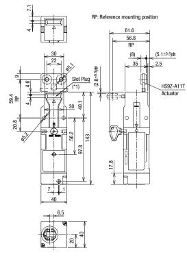
When using angle adjustable actuator (HS9Z-A15T)
